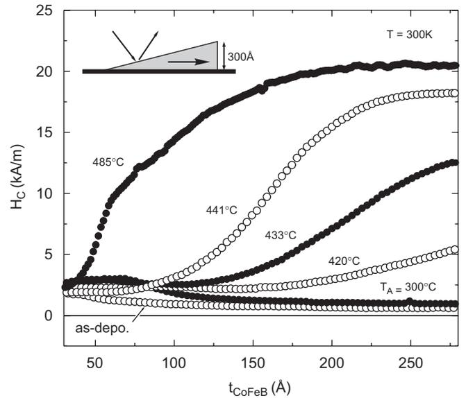
Fig. 2. Room-temperature coercivity ( $H_C$ ) of  $\text{Co}_{72}\text{Fe}_{20}\text{B}_8$  as a function of the film thickness  $t$ , using magneto-optical Kerr-effect (MOKE) on a wedge-shaped layer from 0 to 300 Å. As indicated, the annealing temperature  $T_A$  is varied between 300 and  $485^\circ\text{C}$ .
